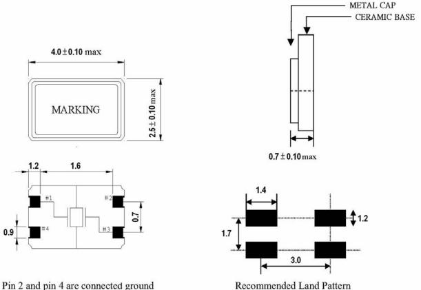
Pin 2 and pin 4 are connected ground
